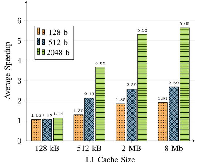
Fig. 4. L1 cache size scaling showing the average speedup compared to baseline cache size of 32 kB for increasing vector lengths
