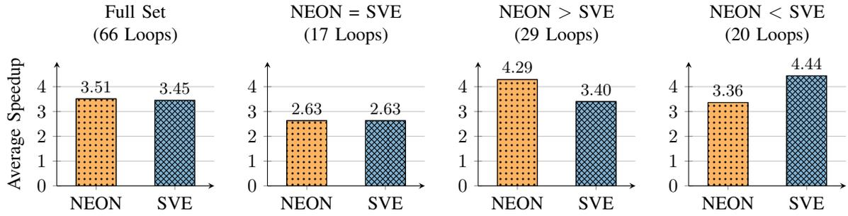
Fig. 1. Speedup comparison of loops vectorized with NEON and vector length agnostic SVE (128 b vector length); average speedup is determined by the geometric mean of individual loop speedups
