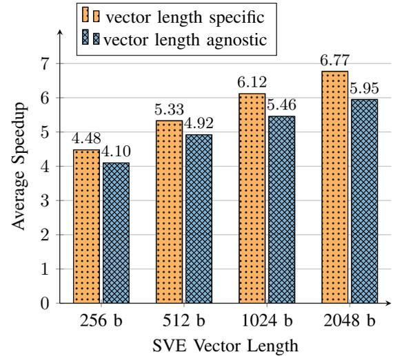
Fig. 3. Comparison of average speedups of 88 loops for VLA and vector length specific code built for varying vector lengths
