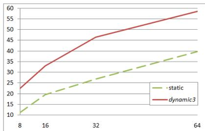
Figure 8. Scalability: A comparison between (100,000;\*; *static*) (dotted line) and (100,000;\*; *dynamic3*) (continuous line). For each algorithm, 100,000 agents are simulated with 8, 16, 32 and 64 workers. Each tests lasts 12,000 simulation steps.  $x$ -axis indicates the number of workers;  $y$ -axis plots the average number of simulation steps per second.
