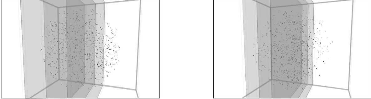
Figure 1. Two snapshots showing 1,000 agents simulated by 4 workers: (left) a simulation step corresponding to a sparse distribution of agents; (right) a dense distribution (middle regions are thinner). These screenshots have been obtained by gathering simulation data on a single worker that performed the rendering. A video is available [5].
