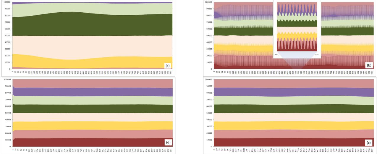
Figure 6. Distribution of agents per worker. Each color represents a different worker.  $x$ -axis indicates the simulation step (1,000 simulation steps are depicted) while the  $y$ -axis represents the distribution of agents. (a) (100,000; 8; *static*) (b) (100,000; 8; *dynamic1*) (c) (100,000; 8; *dynamic2*) and (d) (100,000; 8; *dynamic3*).
