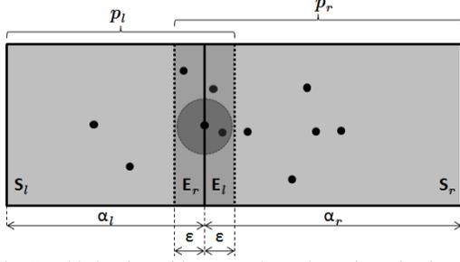
Figure 3. Load balancing with two workers: the main region is partitioned into  $S_l$ , simulated by  $p_l$  and  $S_r$  simulated by  $p_r$ .  $E_l$  (resp.  $E_r$ ) represents the portion of  $S_r$ , (resp.  $S_l$ ) that needs to exchange information before each simulation step.
