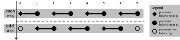
Figure 5. Load balancing with multiple workers. Each worker, after each simulation step, updates, by turns, one of its boundaries. Turns are chosen in such a way that neighbor workers always update the position of their shared boundary at the same simulation steps.
