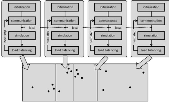
Figure 2. The simulation carried out on 4 workers: upper part the phases each worker executes per step; lower part the main region divided into 4 slices of different sizes, associated to workers.
